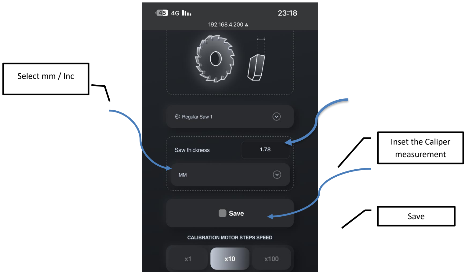
Figure 25: – Save the saw thickness
