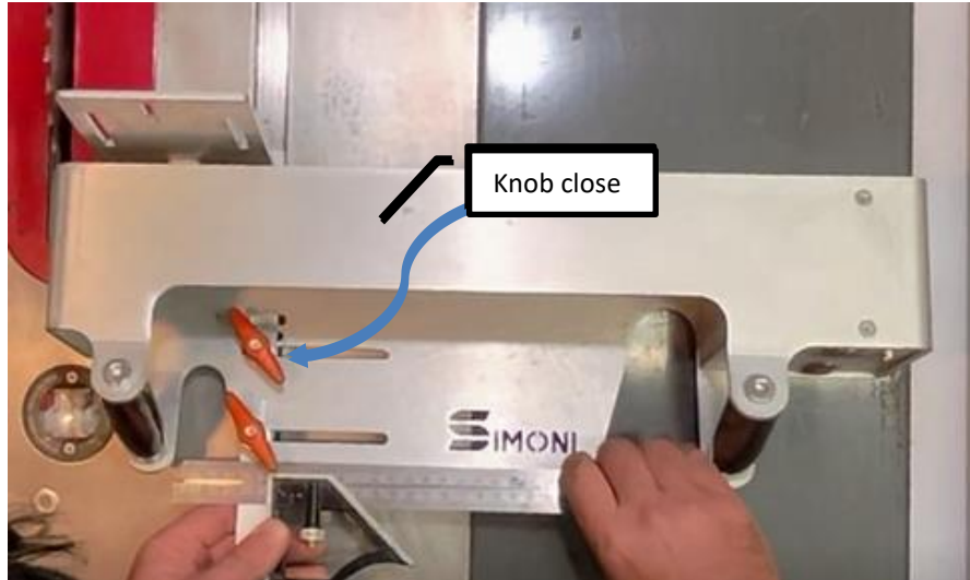
Figure 11: – SIMONI Jig body 90° calibrations done
