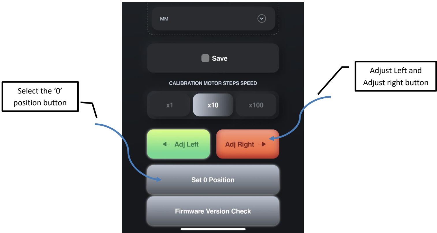
Figure 27: – Zero point, save the calibration point by selecting 'Set 0 Position'
