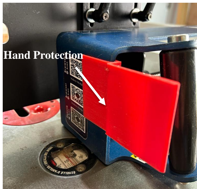
Figure 12: – How to assembly the Hand Protection
