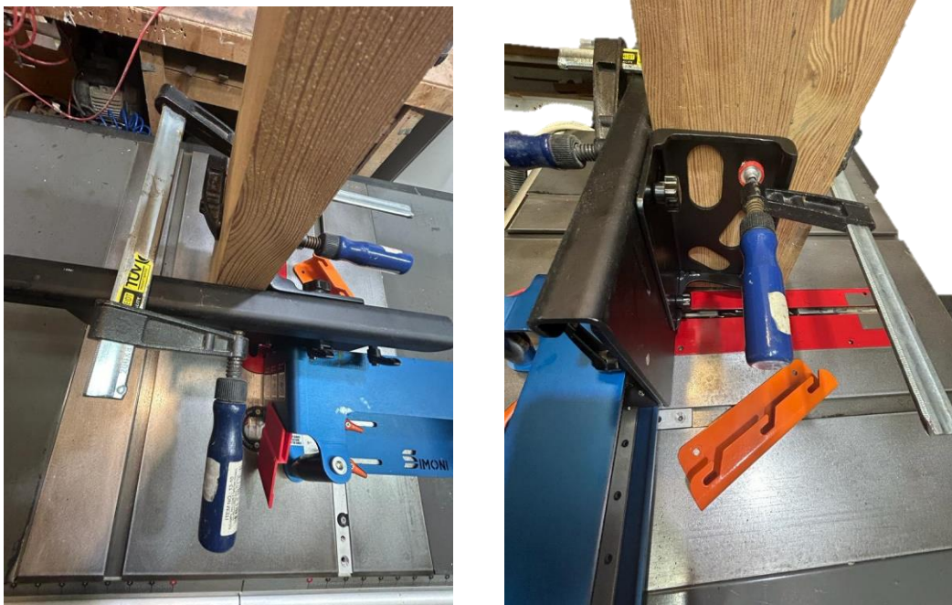
Figure 18: – Correct Clamp, the clamp has wood, change the clamp bar
