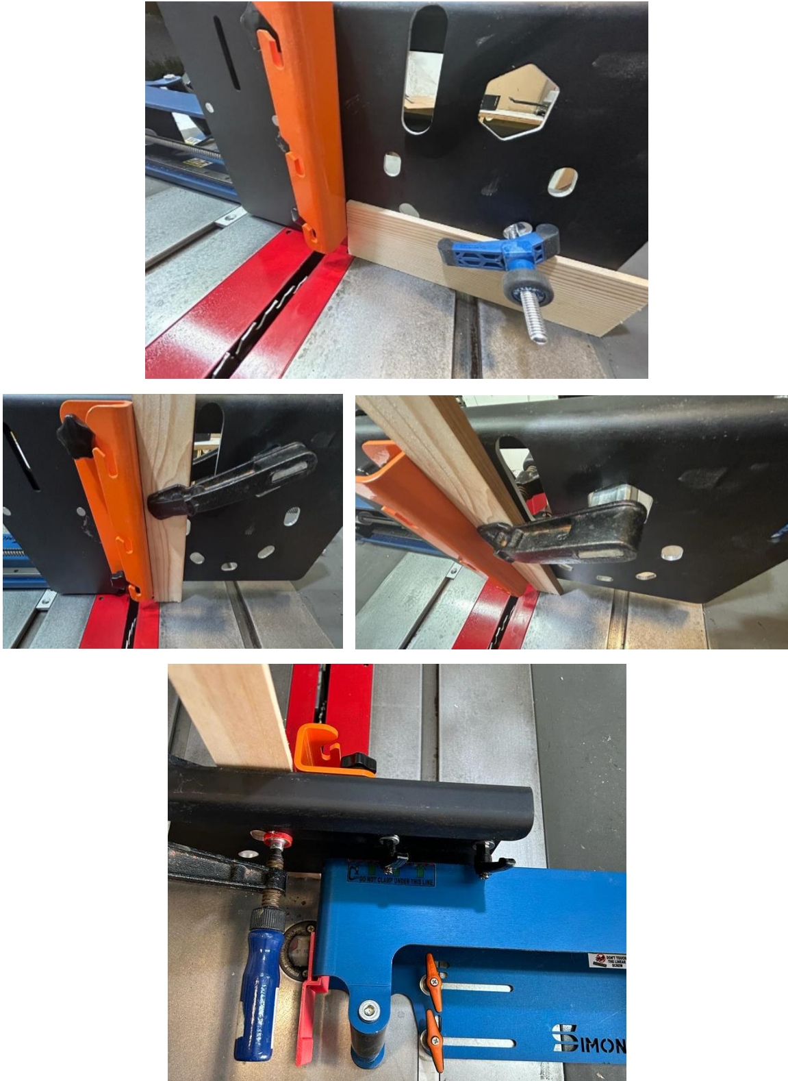
Figure 17: – Correct Clamp, several Method
